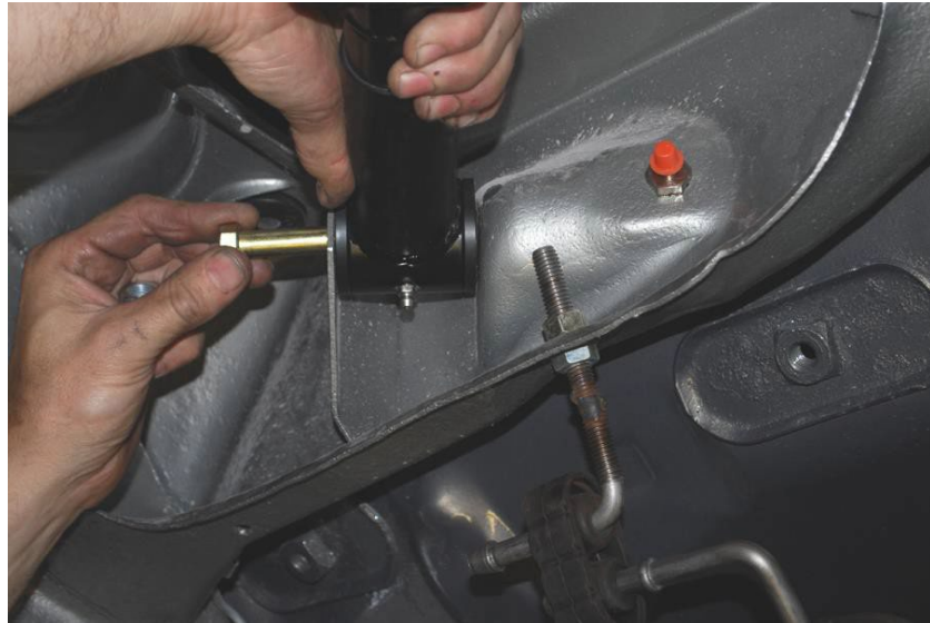
Figure 3: Grease fitting pointing downward
