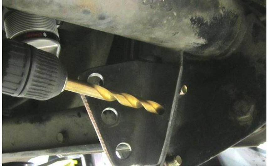
**DO NOT** skip these steps. Both of the 7/16" bolts must be installed to properly secure the coilover conversion bracket.
