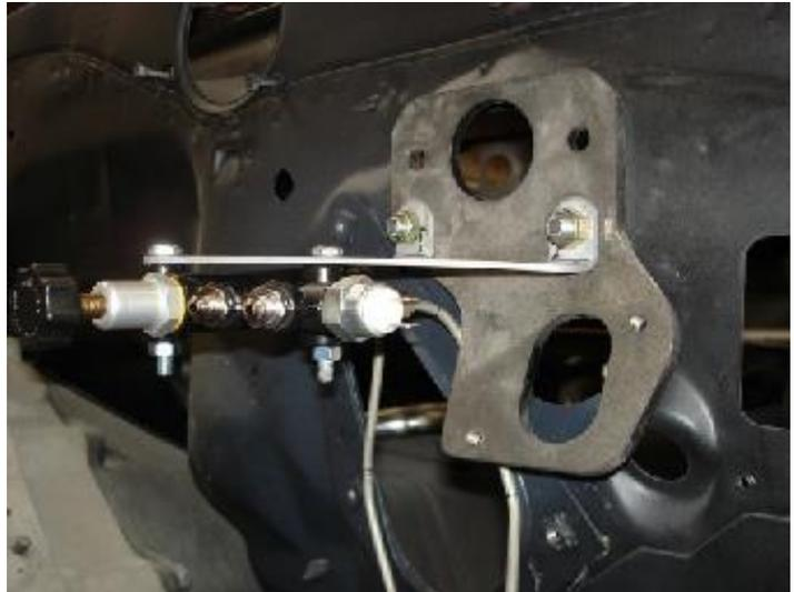
**NOTE:** We have **NOT** supplied brake lines that go from the master cylinder to the proportioning valve. This is due to variations in fittings and master cylinder designs. The easiest way to complete the connection would be to use braided flex lines that you can purchase from a performance parts retailer. If you have the proper tools, you can fabricate custom hard lines.
