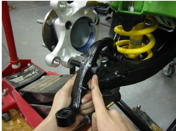
**Note:** The Speedtech spindle requires a C5/6 based brake package to be installed. We recommend Baer or Wilwood brakes. Follow manufacturer's instructions for your specific brake system. Be sure to properly bleed the brakes before driving the vehicle.
