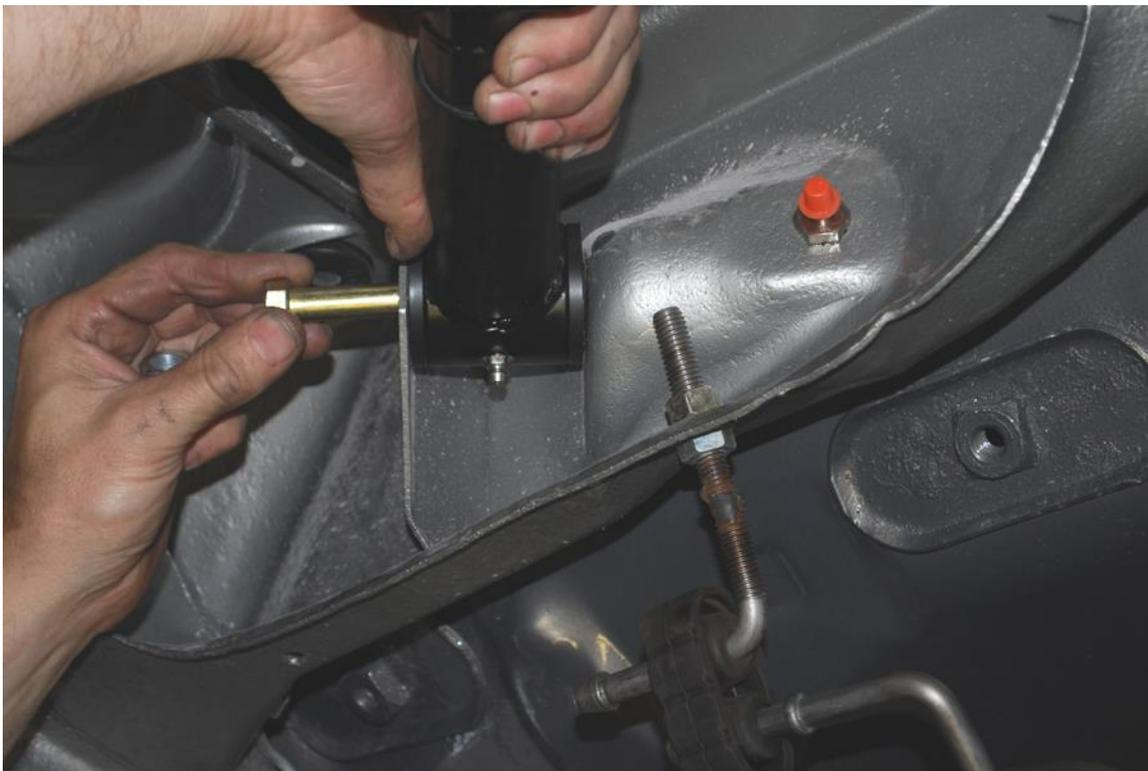
5. Remove the factory lower trailing arms. Adjust the Speedtech lowers as needed in the same manner as the uppers. Install the trailing arms with the new bolts. Raise the axle to ride height and recheck pinion angle. If the angle is off, remove the rearward end of the lower trailing arms. Adjust the driver's side arm and reinstall. Adjust passenger arm to match bolt hole alignment and reinstall. Check pinion angle again. Repeat process until desired pinion angle is achieved.
