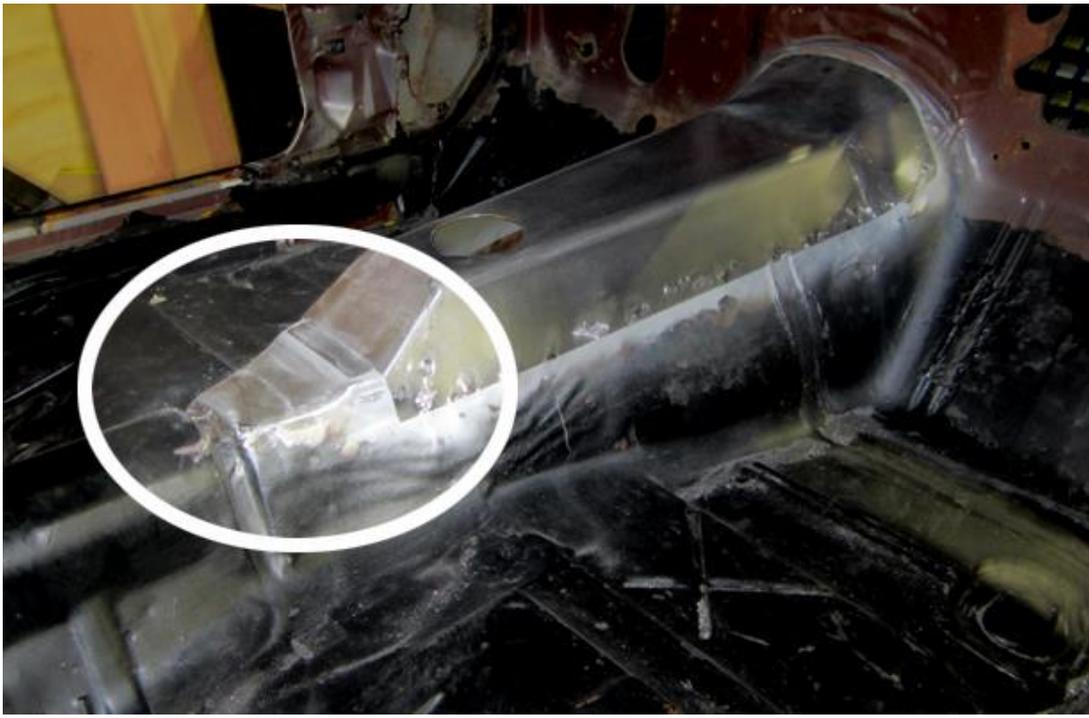
6. Once the cover is properly and securely fastened to the floor, be sure to seam seal all areas on top *and* underneath where the tunnel cover meets the floor.
