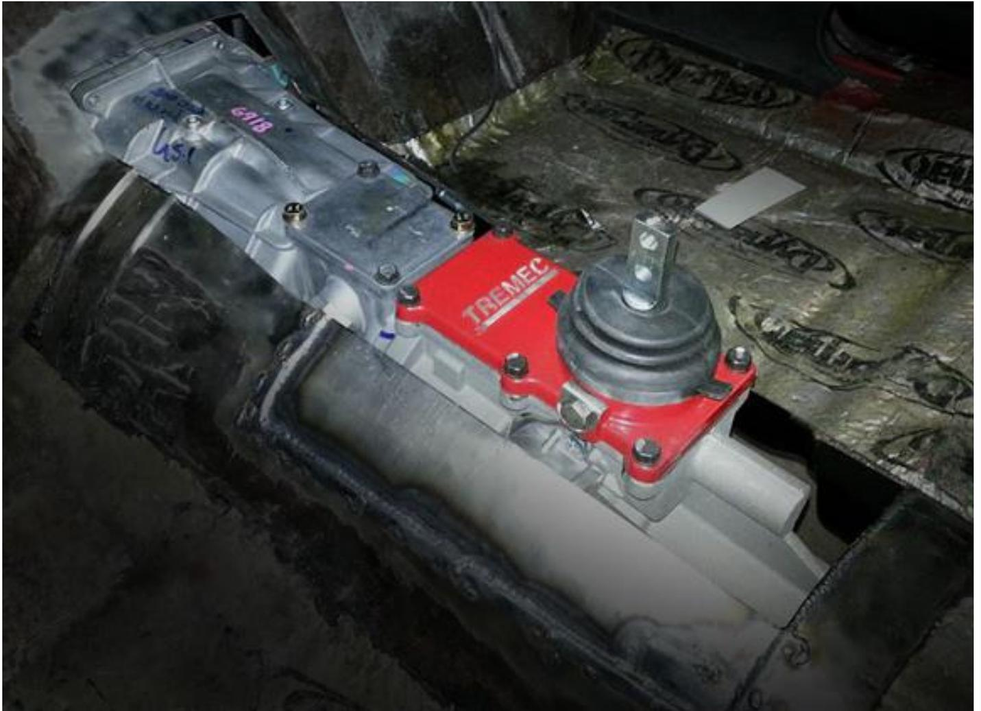
4. Factory floor shifted Camaros will need the shifter hump removed and a piece of sheetmetal attached in its place to seal off the rest of the tunnel. See below.
