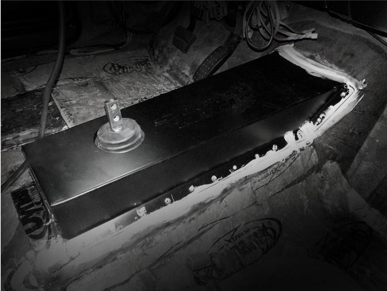
7. As the inside of the Tunnel Cover and the area of the floor pan covered by the Tunnel Cover may be exposed to outside elements, we recommend protecting these areas with a high quality paint or other surface protector. Attach the Tunnel Cover securely to the floor. We recommend using a high quality seam sealer on areas where the Tunnel Cover makes contact with the floor pan, and in any area where there may be flange gaps because of floor pan shape.
