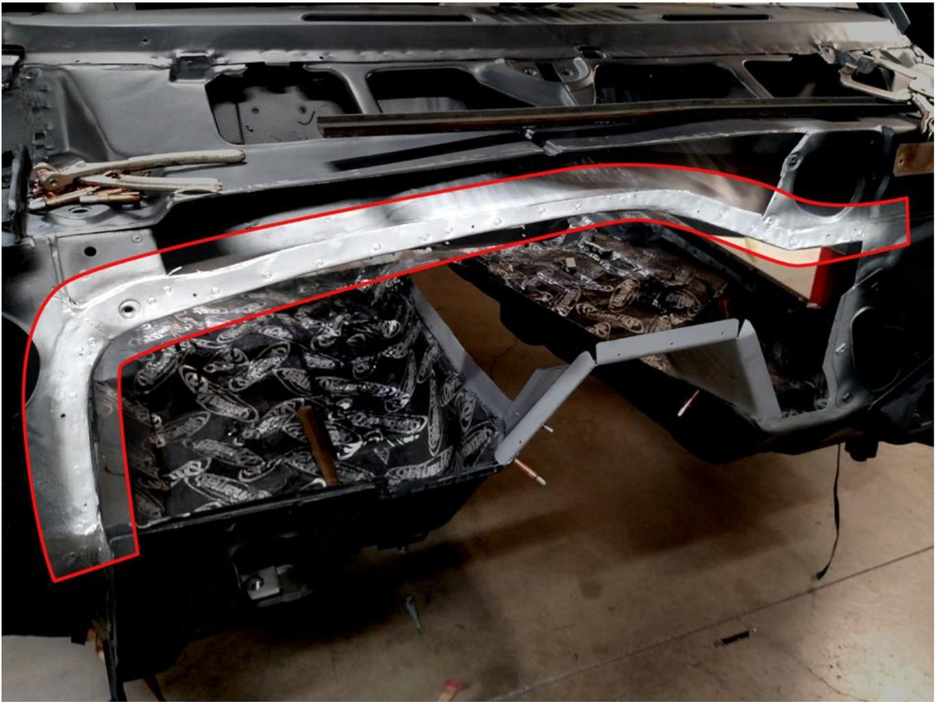
**4.** Proceed to cut along your marked cut lines and remove the old firewall. Mock up your new firewall in place. You can hold it with sheetmetal screws, clocos, etc.
