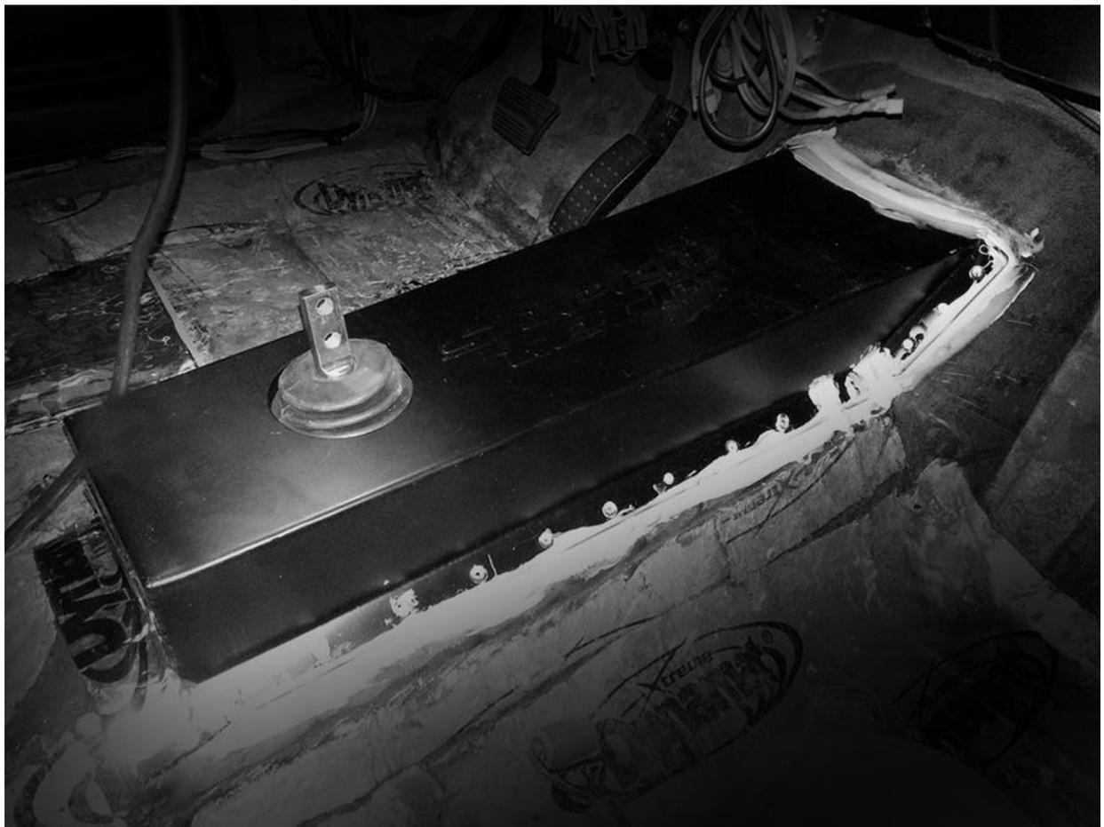
**7.** Cover your tunnel cover as fits your needs. We recommend splitting and securing vacuum tubing around the diameter of the shifter hole to prevent
