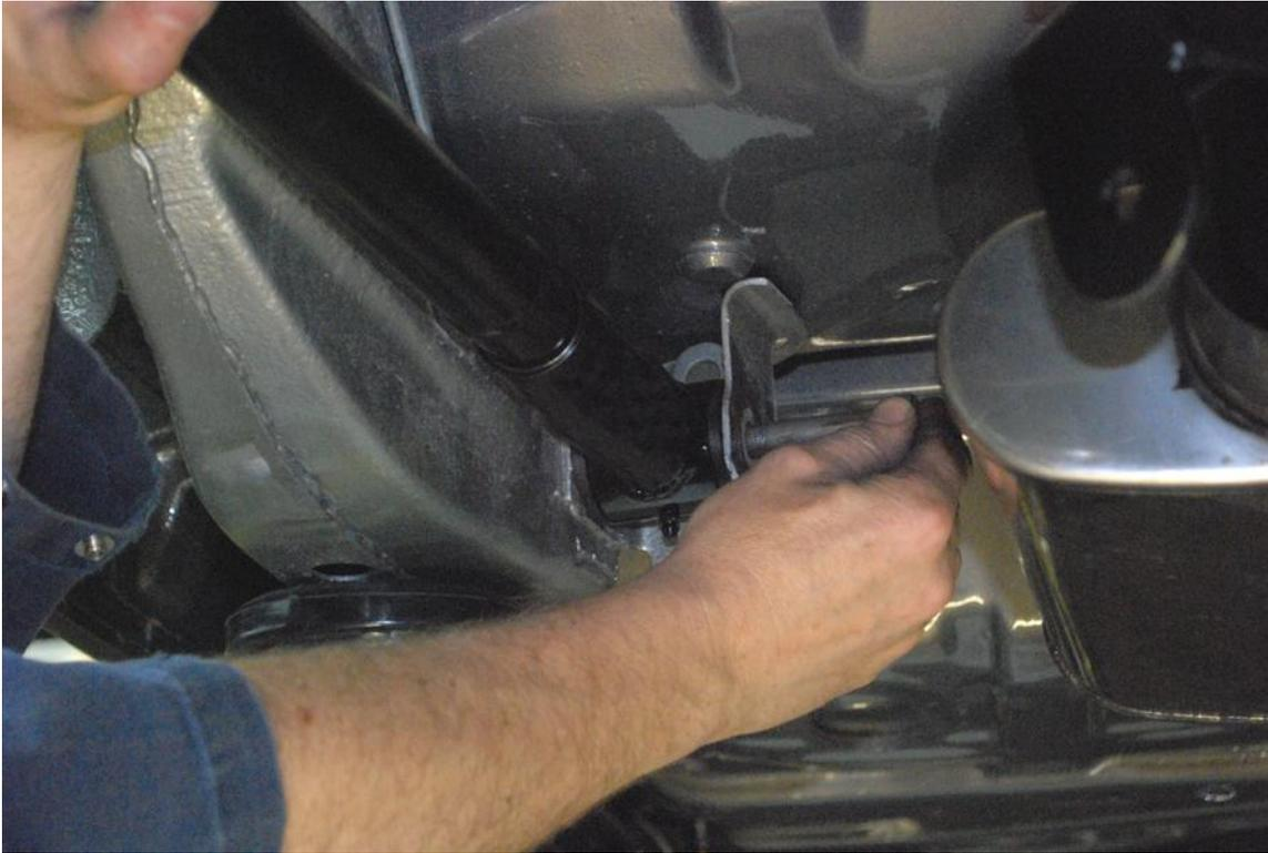
6. Check to make sure the rear axle is laterally centered side to side in the car and the wheels are centered front to back in the wheel opening. Adjust trailing arms as needed. Always be sure pinion angle is rechecked as centering adjustments are made.
