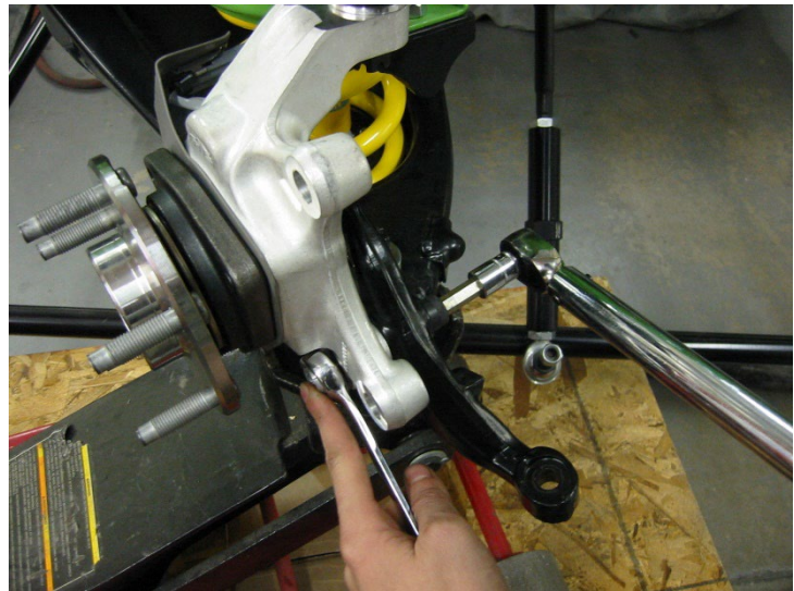
Figure 6: Two images of factory steering arms
