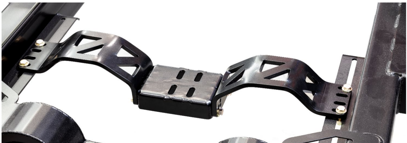
Figure 18: Installing the crossmember onto the frame
