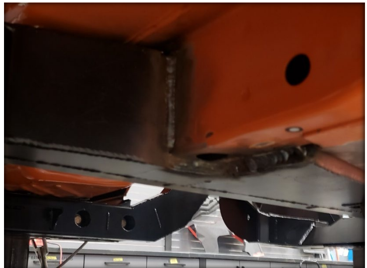
Figure 16: Where spot welding in the cab must be completed
