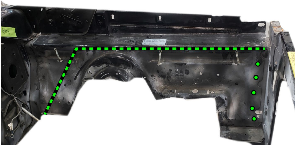
Figure 19: Marked crease where the inner fender can be removed
