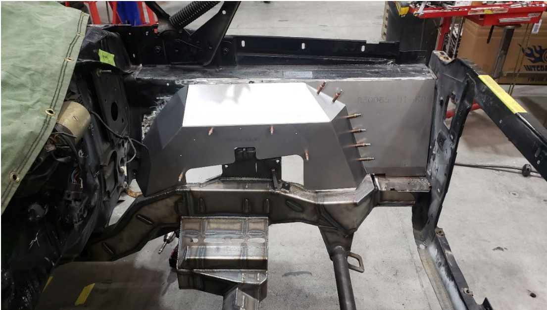
Figure 20: Adding the rear tub to the old fender
