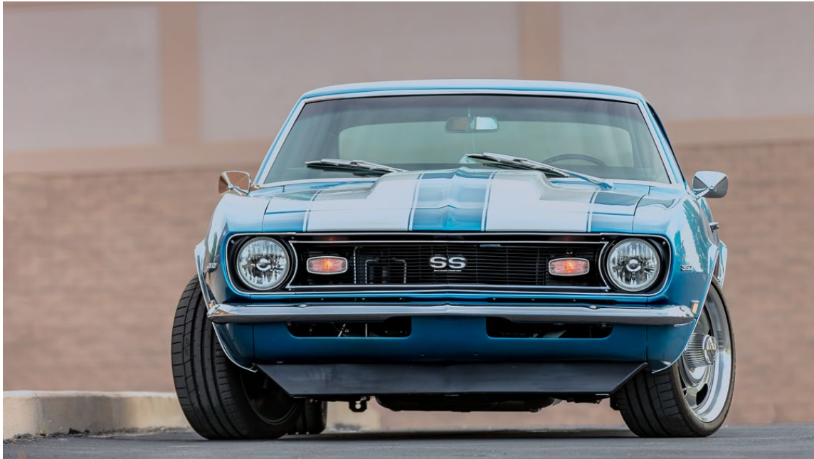
Figure 1: 1968 D8nite Camaro features our GT front suspension and torque arm rear suspension
