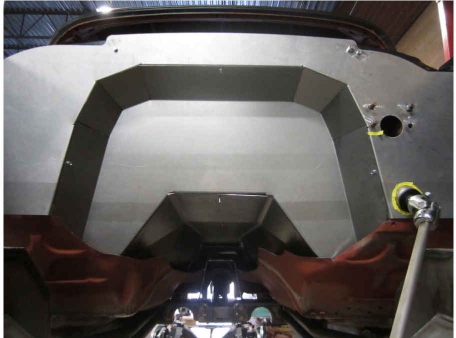
Figure 6: Drilled hole for brake pushrod
