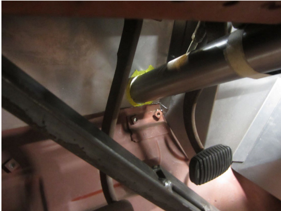
Figure 8: Steering column in relation to the factory bracket
