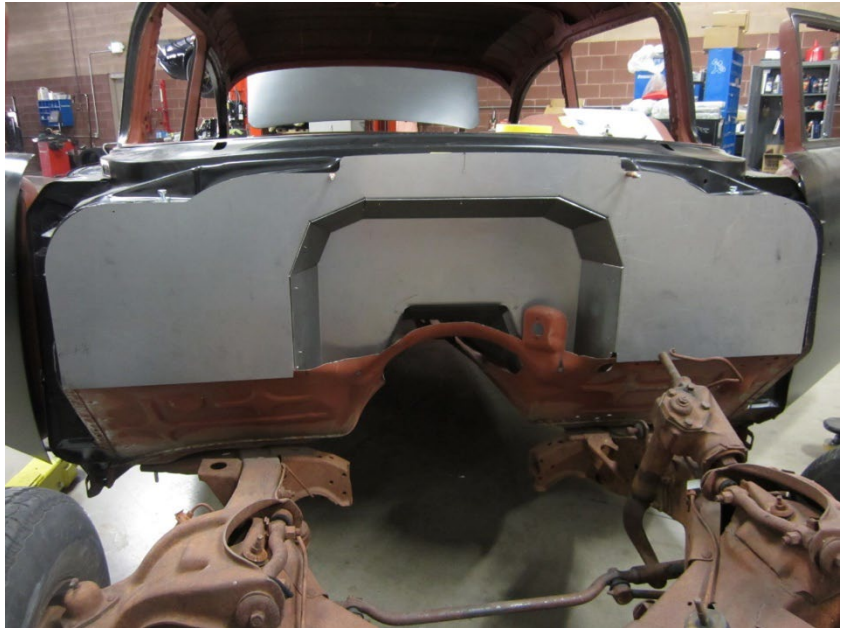
Figure 4: Bellhousing to firewall transition in place
