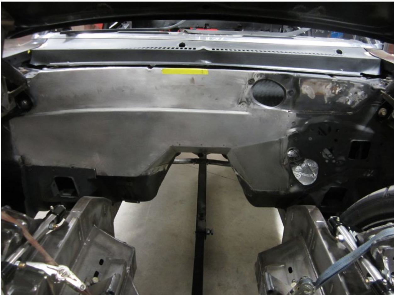
Figure 6: Welding the firewall in place
