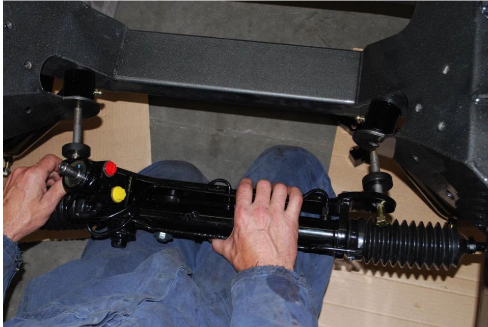
Figure 6: Two mounting bolts entering the subframe
