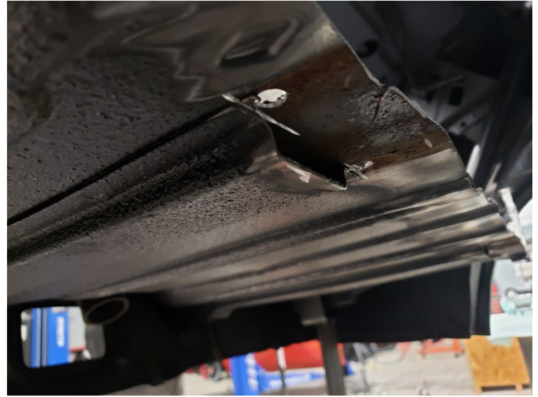
Figure 6: Marking the frame rail 3" back from rear cut line
