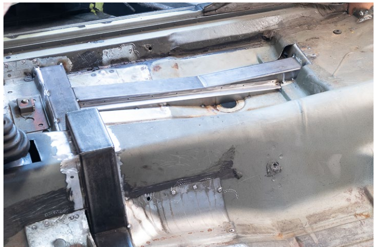
Figure 14: Installing the subframe connector
