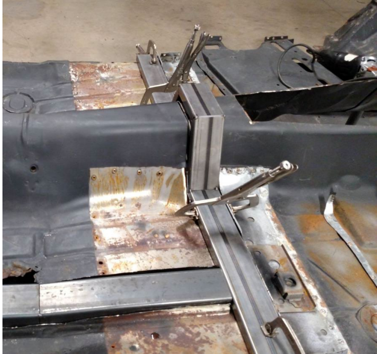
Figure 12: Crossmember set down on top of the pan
