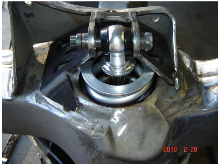
Figure 9: Mockup of the upper mount
