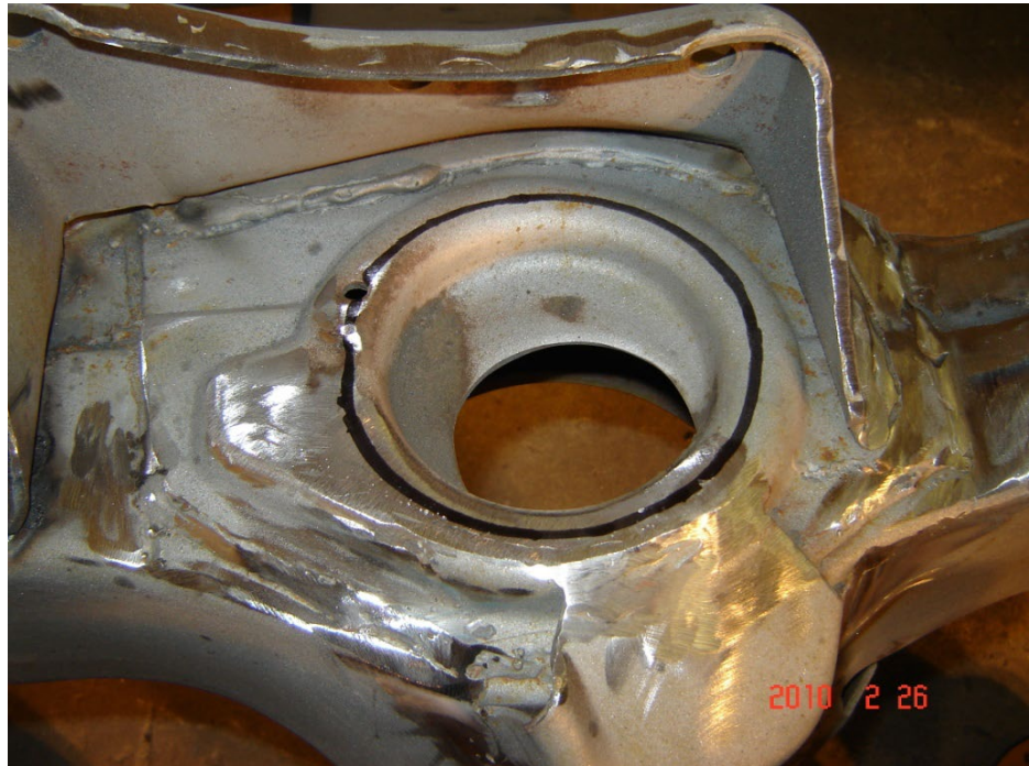
Figure 5: Cut line for the inner spring cup
