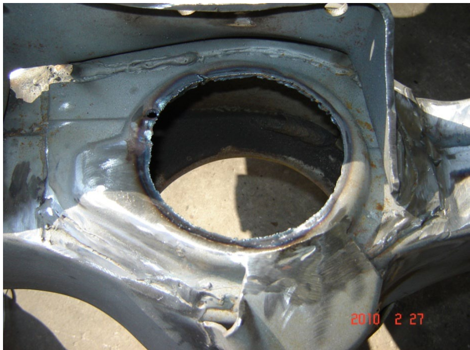
Figure 6: Final product after cutting the inner spring cup
