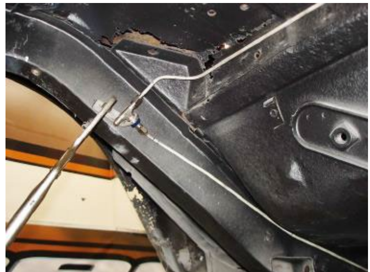
Figure 11: Inserting a bulkhead "T" through the mounting bracket
