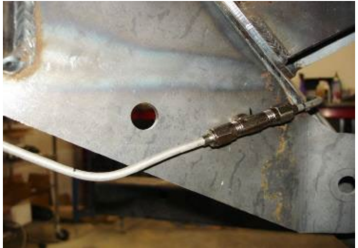
Figure 7: Driver's side bulkhead T installed with both lines connected
