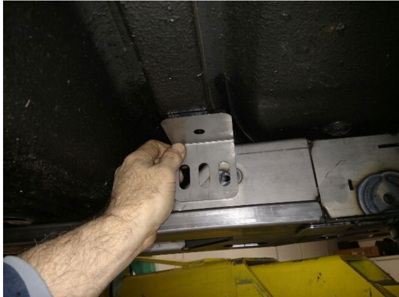
Figure 3: Location of where the bolt goes
