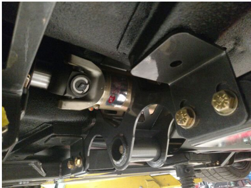
Figure 6: Front L bracket locations
