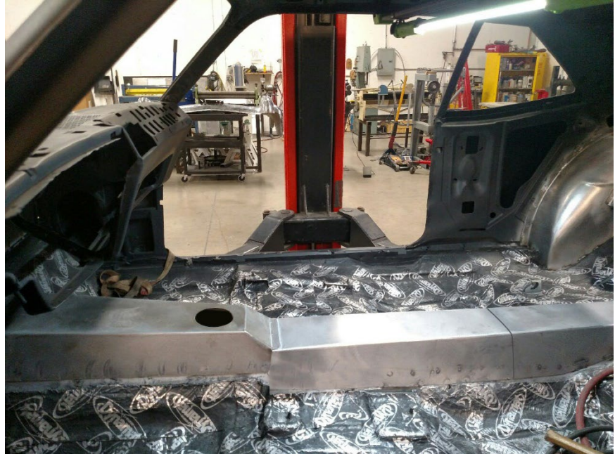
Figure 9: End result of floor tunnel
