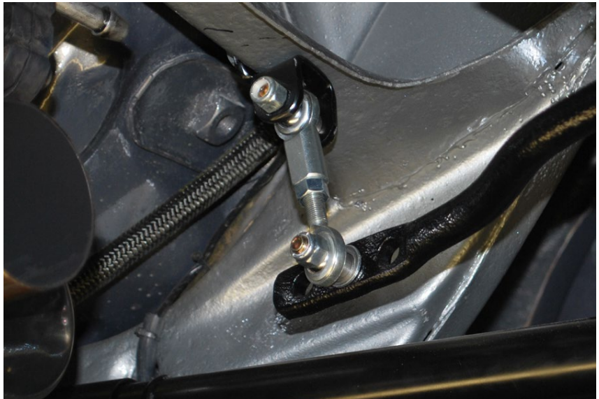
Figure 6: Two images of bolting the trailing arms and sway bars
