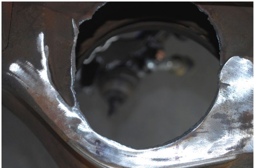
Figure 6: Final product after cutting the inner spring cup
