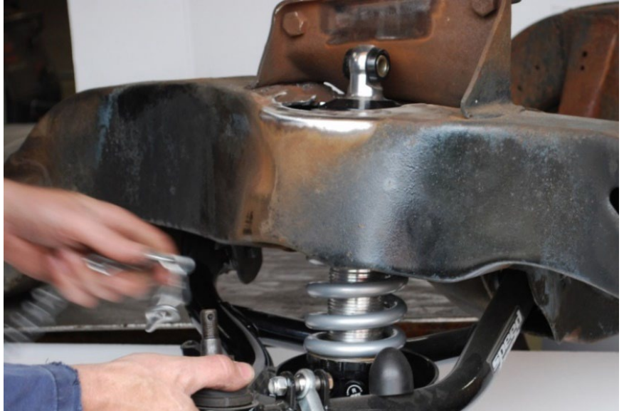
Figure 8: Mockup of the lower mount
