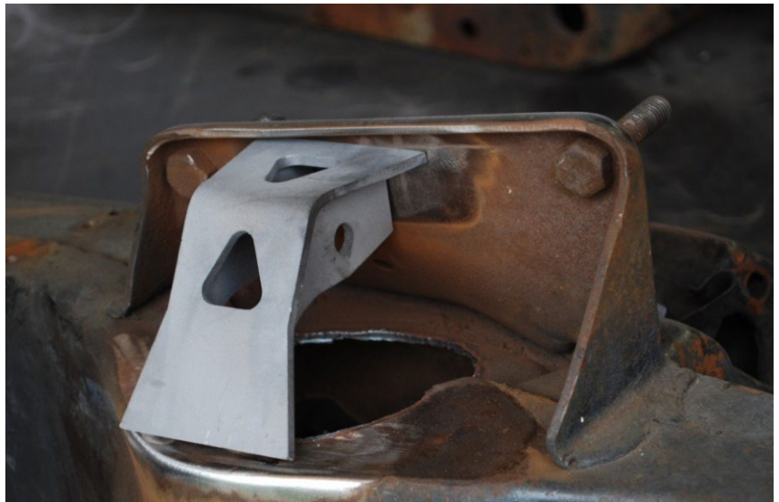
Figure 9: Mockup of the upper mount
