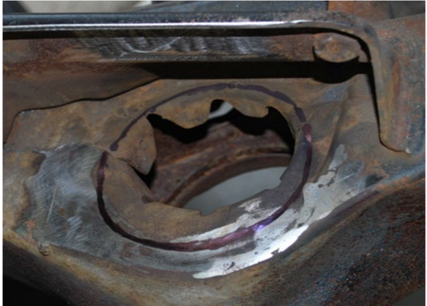
Figure 5: Cut line for the inner spring cup
