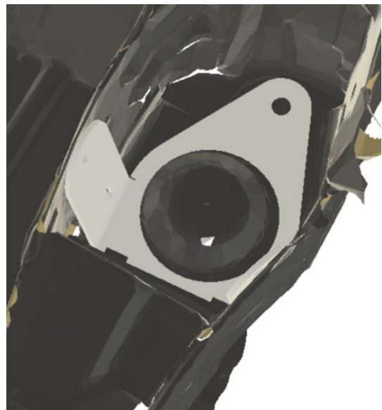
Figure 3: Two images depicting the upper shock bracket
