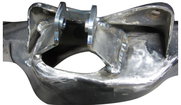
Figure 10: Chicane upper bracket
