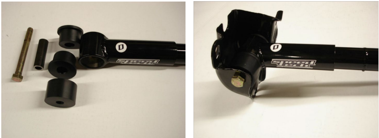
Figure 15: Two images depicting the spring pocket and trailing arm assembly
