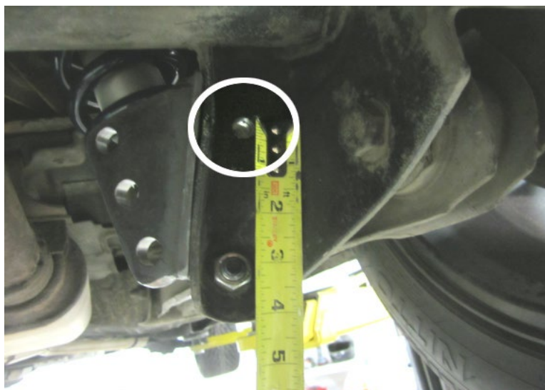
Figure 5: Measuring the rear side of the factory bracket
