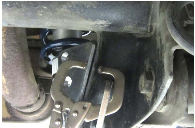
Figure 4: Clamping the bracket to the factory mount
