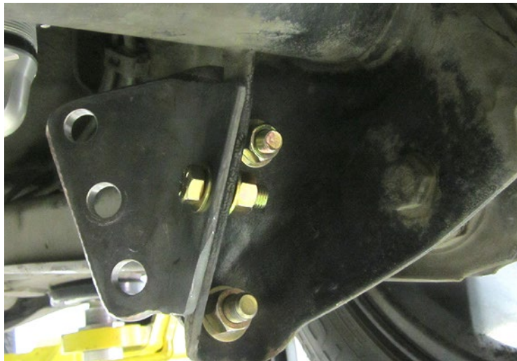
Figure 7: Bolting the coilover conversion kit
