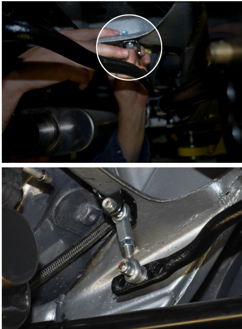
Figure 5: Two images that depict the bolting of the end links
