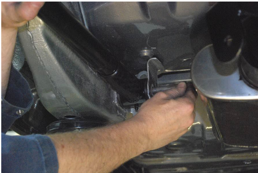
Figure 4: Lowering the trailing arms
